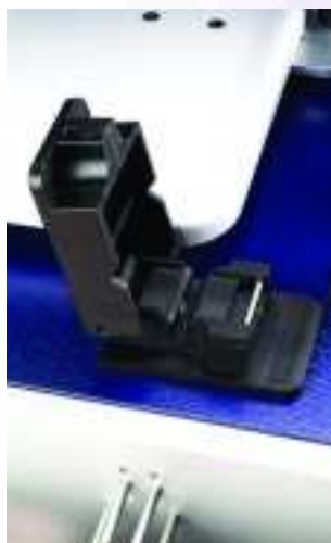
Top sensor for top/top red cell and air detection.
